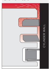
10% of the gas-tight seal is due to the piston ring's own elastic force and 90% to the actual combustion pressure.
