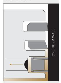
The bottom piston ring, the oil scraper ring, provides a nice thin layer of oil on the cylinder wall.
