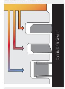
The top piston ring, the compression ring, makes sure that most of the heat is dissipated.
